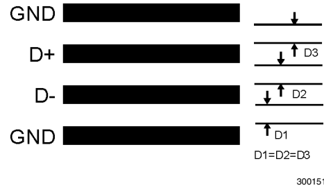
FIGURE 9. Ideal Diode Trace Layout
